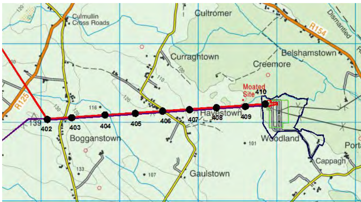
Figure 2.6: Addition of a New Circuit along Towers 402 to 410 of the existing Oldstreet to Woodland 400 kV OHL in the MSA
